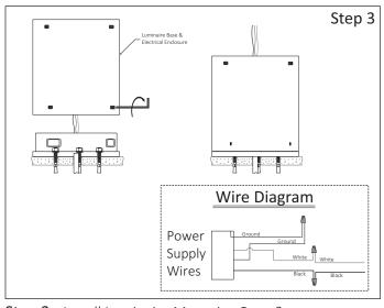
Step 3 - Install Luminaire Mounting Base & Make Wiring Connections:
