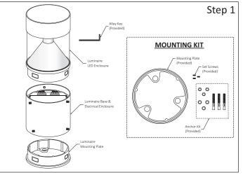
**Step 1** - Disassemble Luminaire Parts for easy Installation: a.- Remove Luminaire Mounting Plate from Base.
