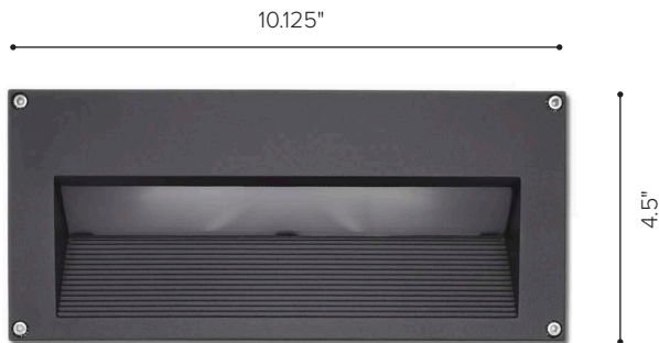
SLS650 powder coated faceplate glare-hood over impact-resistant glass diffuser
