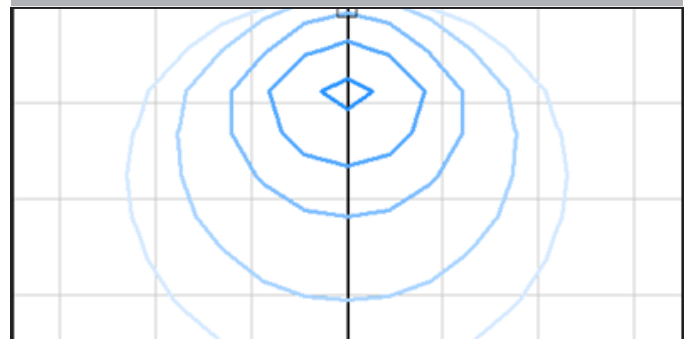
Foot-candles: 0.1, 0.2, 0.5, 1 | Grid spacing 5'
