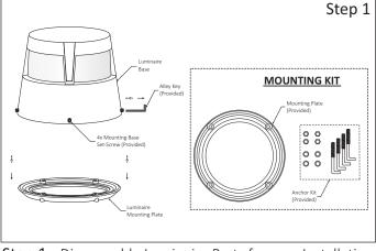
Step 1 - Disassemble Luminaire Parts for easy Installation: a.- Remove Luminaire Mounting Plate from Base.
