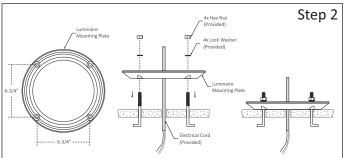
Step 2 - Install Luminaire Mounting Base:
