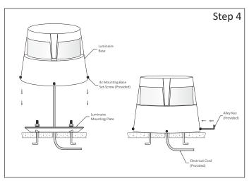
Step 4 - Install Luminaire Base:
