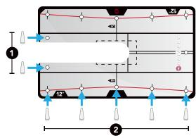
\*\* When installing pegs, insert from the bottom of the mirror, up. The peg will slide up through the hole and will remain snug throughout use.
