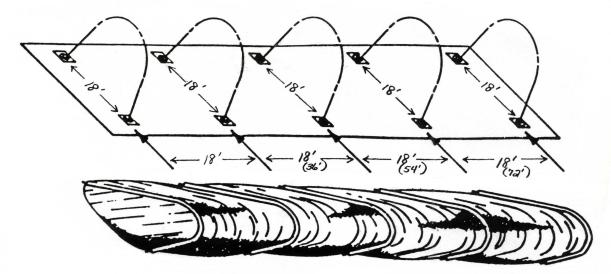
Each arch assembly will have a natural spread greater than 18'. Legs will have to be brought in to the 18' width.
