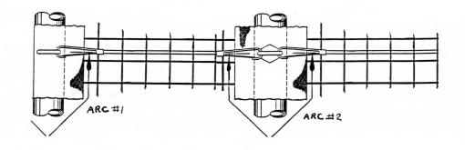
Now snap the remaining 18' ropes to the eyebolts at the side Velcro flap openings. Snap the ropes on the outside of the cage and run the cable under the net (or inside the cage) to the next arc. Weave it through the net and again snap the rope to the eyebolt outside the arc as you did in the above paragraph.
