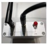
On the device, remove the red plastic from the "wifi-BT" input, and connect the wifi antenna
