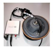
Remove the red plastic for "GNSS" and connect the smaller end of the satellite antenna cable. (sma-male connector)
