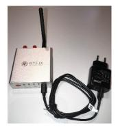
Plug in the usb-c cable and power the device with any usb charger with at least 1amp. (Also, a regular phone charger works)
