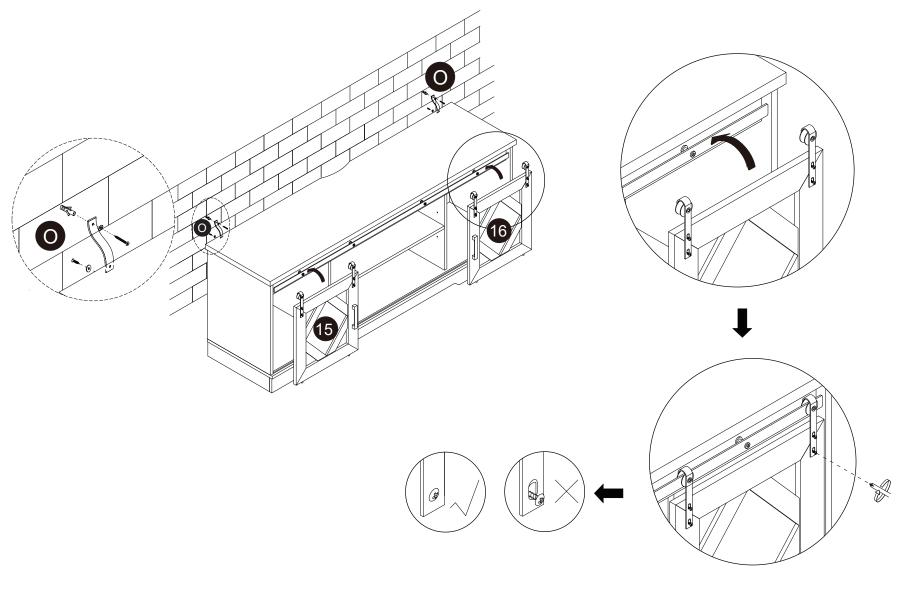
After installing the doors (15, 16) in position, adjust door height and leveling, then fix screws tight and slide doors (15, 16) into designated area.
