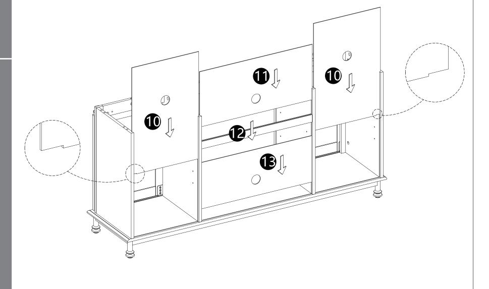
·Carefully slide panels (10,11,12,13) into place along the back of the assembly.
