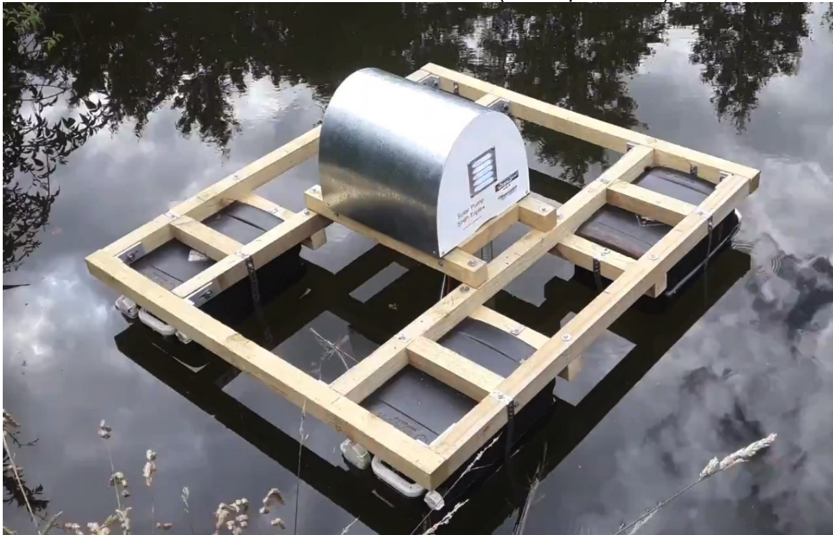
React pump pontoon mounted
