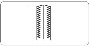
Simple zigzag stitching is used to finish raw edges (overcasting) on most fabrics in order to prevent fraying. This is the fastest way to finish an edge.
