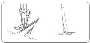
Pin or baste zipper tape to fabric and place it under the
