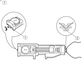
With the buttonhole foot with slide raised, hook the filler cord on the cord pin at the back of the buttonhole foot with slide.
