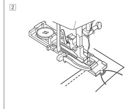
2 Lower the needle into the garment where the buttonhole will start and lower the foot. Depress the foot control gently and sew the buttonhole.
