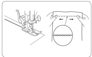
The stitch is sewn with two forward stitches and one reverse stitch, creating a seam that is difficult to tear.
