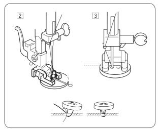
Match the holes in the button with the horizontal slot on the presser foot.
