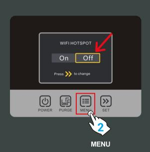
After pressing the "POWER" button to return to the main interface of LCD display, hold down the "PURGE" and "MENU" keys at the same time for 3-5s. The interface will give out a prompt sound, then Wi-Fi icon in the upper right corner will keep flashing.
