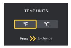
"Temp Units  $^{\circ}F/^{\circ}C$ ": Used for temperature scale switching.Press the ">" button to switch  $^{\circ}F/^{\circ}C$ , after switch symbol of corresponding parts is also changing.
