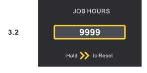
"Indicates":Do I need to clear out this time?", press ">"if you need to clear. When the operation is completed, the working time of the main interface and the working time of this interface will be reset and started to be instant again.
