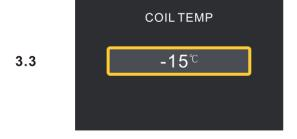
"Coil Temp  $000^{\circ}$ C": Used to display the current temperature of the coil.When it is below zero, the "-" symbol is displayed in front. "-" is not required on zero.
