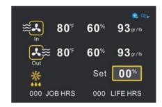
When the user is operating in the submenu, the machine is in the frosting state. At this point, the frosting interface displays 3 seconds, and returns to the submenu program in the background countdown. When the user returns to the main interface without any operation, the frosting state is displayed in the main interface in the way of icon flicker.
