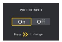
Wifi hotspot: factory setting is "0FF", press > to enable wifi hotspot and switch ON/OFF. The device can transmit data and receive APP commands. The icon flickers when connected on the main interface. After successful connection, the icon displays normally.
