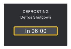
When the machine is running normally, "Deffrost SHUTDOWN IN 06:00" will occurs in the interface after defrosting. It's defrost countdown use seconds as units. This screen displays only 3 seconds. Displays the previous interface and status after restoration. If it is the home screen, the frost icon will flash.
