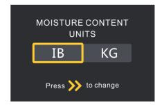
"MOISTURE CONTENT UNITS": It is used to switch the unit of GPP value with moisture content. Press > to switch the lb or Kg, after switch symbol of corresponding parts is also changing.
