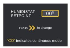
"Humidistat Setpoint 00%":Used for setting dehumidification mode humidity.Press ">" to set the humidity. The adjustment range of humidity setting is between 25 and 80%. Each key rises or falls 5%, which can be recycled.
