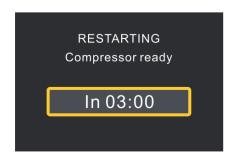
"Compressor ready IN 03:00" indicates: That the interface will be displayed when the compression is in a protected state. (including power-on and shutdown, the humidity rises immediately after the arrival of LO HI, and the shutdown resumesimmediately after the emergence of LO HI). Displays the countdown in seconds. If the above situation does not occur within 3 minutes, it is not shown.
