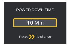
The power down time is adjusted according to">" and the power down time increases from 3 to 20 minutes (3-5-10-15-20), which is the so-called stop time of the fan after shutdown, in order to better drain the water.Factory set for 3 minutes. (the other state of the fan is still 15 seconds.)
