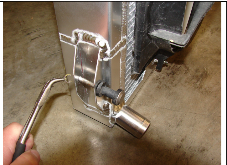
Install the bottom radiator support from your OEM system. Sometimes it is required to install this support with the system already in the car. Some users have used bolts instead of the factory hardware and others use only the top mounts. I run the factory hardware as shown on my personal car.
