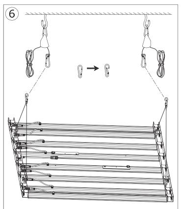
Attach steel ropes to adjustable ratchet hangers.
