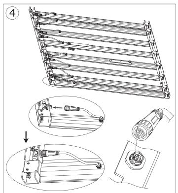
Insert the male connectors (connected to the light bars) into the female connectors (mounted on the frames), and securely fasten the locking rings by rotating them tightly.
