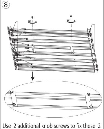
Use 2 additional knob screws to fix these 2 brackets.
