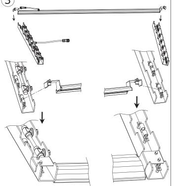
Place the two frames parallel to each other with a distance of 41 inches (105cm) on a flat table, and click each light bar into the frames one by one.
