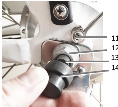
Figure RR4. Correct installation of rear axle into fork. View from bottom UP.
