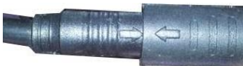
Figure RR5. To re-install rear wheel, follow steps shown in Figure RR3, RR2 and RR1 in reverse order. Make sure the wheel is installed safely. When re-connecting the male and female motor wire, first make sure that both arrows on the wires are aligned, then push both cables together all the way as shown in this figure.
