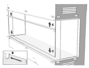
**F:** With the front glass tilted rearwards pull the side glass side forwards. Finely position the front and side glass panels to give the best possible fit and finish making sure the front glass glides back with ease and depresses the micro switch arm on the underside of the heat housing.
