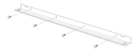
Position the fire on top of the bottom bracket making sure the corner bolts fit through the slots either side and can screw into the underside of the fire. With the top bracket attached to the fire, mark across its length and into the slots above each hole on the back edge. Remove the fire, remove the top bracket and 13mm screws from the fire and mark the holes on the wall, drill and fit the rawl plugs using an M10 bit. Using the 60mm screws fix the bracket to the wall.
