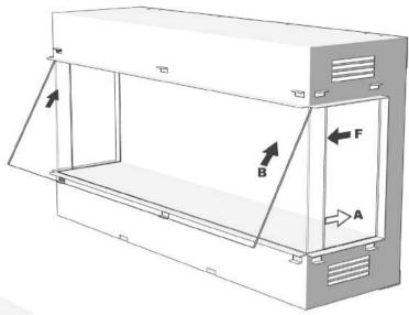
**D:** Slide the handle along the top right hand side of the glass.
