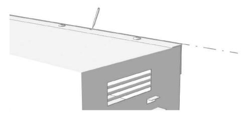
Slide the fire into the channel created by the top and bottom brackets. Screw the top bracket back onto the fire with the 13mm self-tappers and bolt each corner of the bottom bracket threw the slots either side into the fire using the M6 bolts and washer supplied. At this point you will be able to level the fire accordingly at the base by loosening and tightening the bottom bolts.
