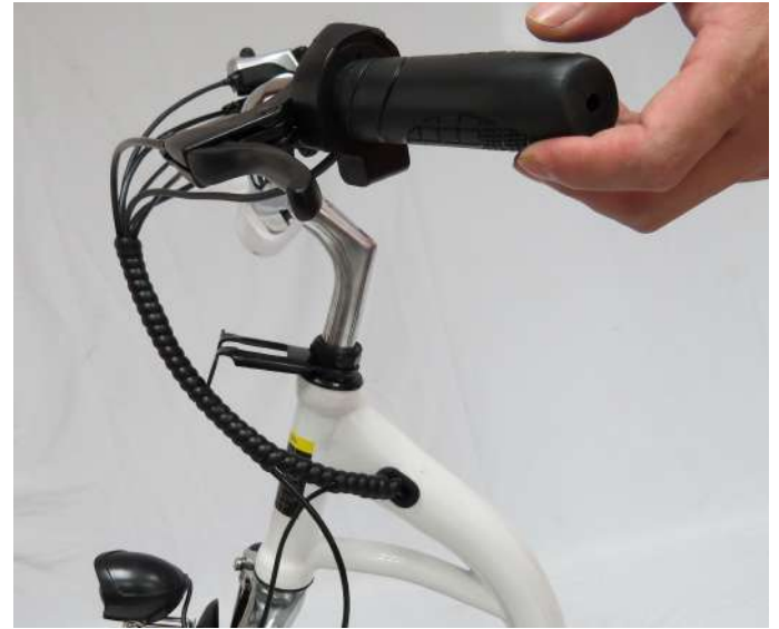
Adjust the Height and Handlebar Alignment Relative to Wheel
