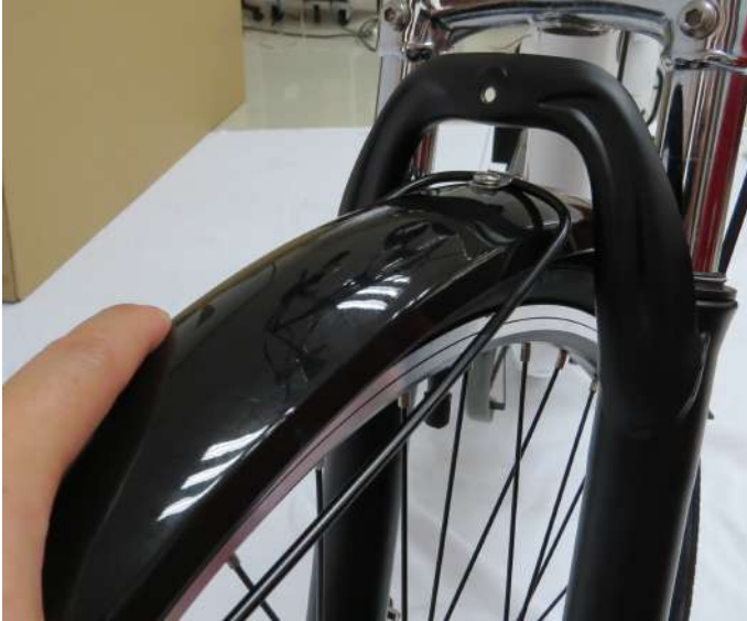
Installation of the Fender
