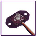
The Light sensor bit almost looks identical to the LED bits, however, the sensor called a 'phototransistor' has a water clear lens.
