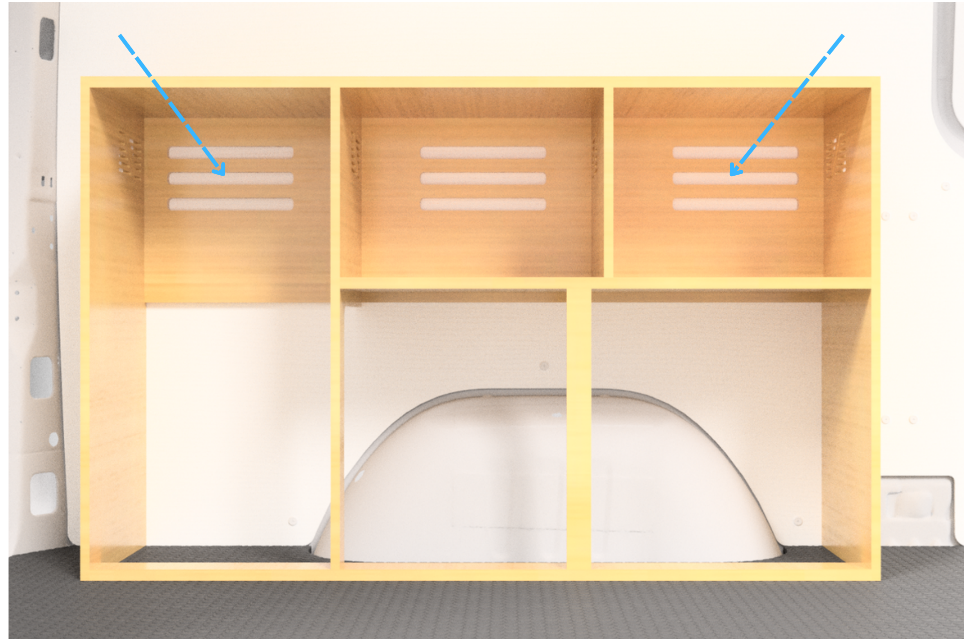
Rear panel factory holes example.
