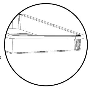
These Trim Rings must be fastened properly to the walls of the vehicle to avoid damage or injury. You are responsible for ensuring that this product is fastened using rivet-nuts or other fastening method equal in strength. Modification to this unit may affect the structural strength of the unit. Avoid making large cuts on ring walls as this may weaken the ring strength. You are responsible for ensuring proper wiring and insulation when wiring your build as faulty wiring may create a fire hazard.
