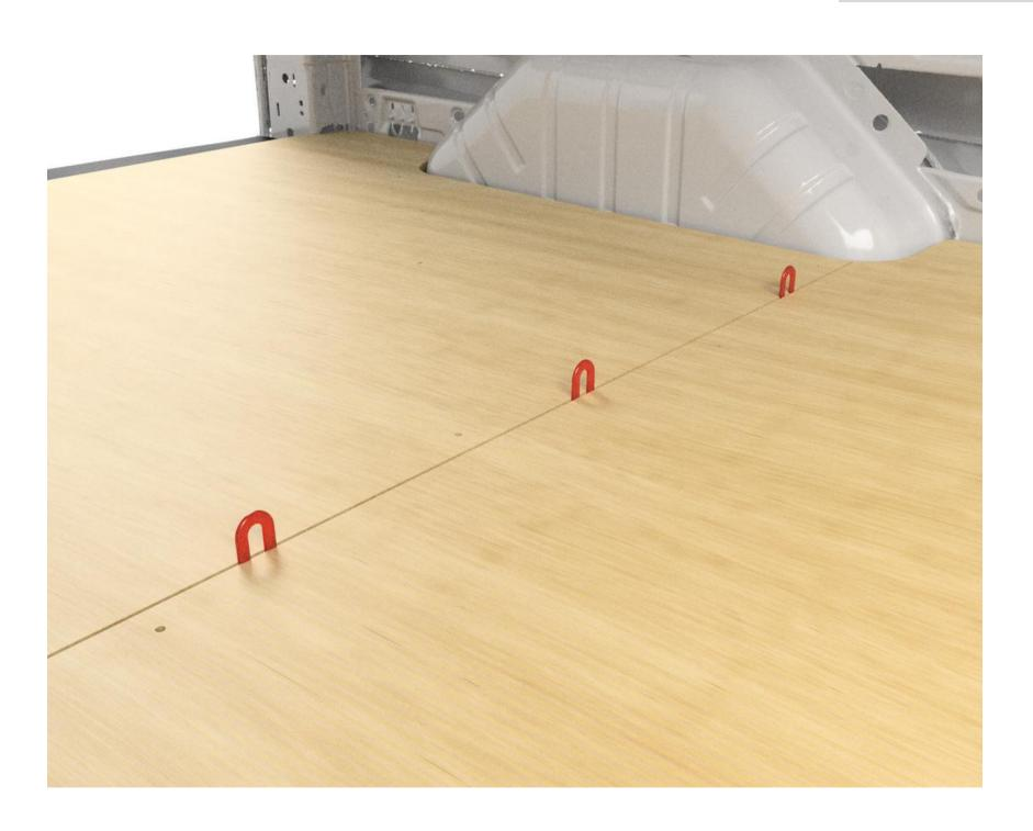
**Note:** The shims are specifically designed to accommodate the expansion and contraction of the subfloor panels. These panels should not be contacting one another during installation.
