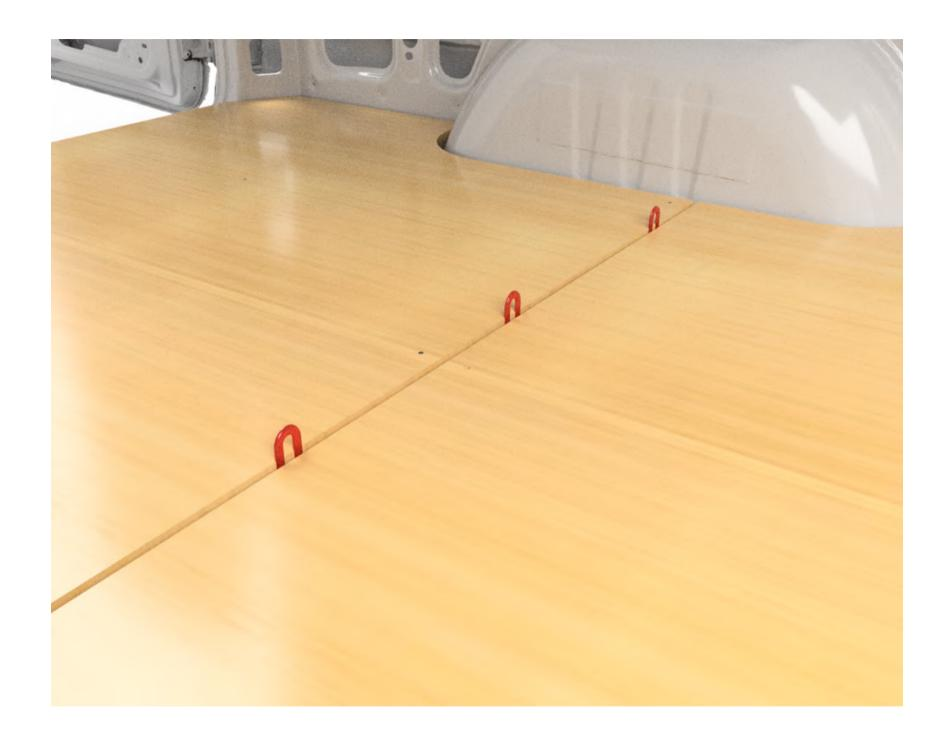
**Note:** The shims are specifically designed to accommodate the expansion and contraction of the subfloor panels. These panels should not be contacting one another during installation.
