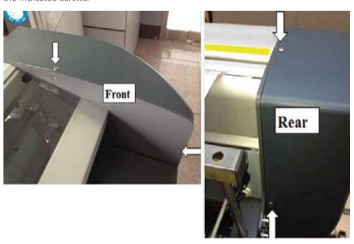
2. Remove the two screws (pictured below) to adjust the height of the limit switch so that the limit switch will make contact with the cutting mechanism. The limit switch should click when its engaged by the cutting mechanism, which will shut off the motor when the blade has reached the end of the machine.
