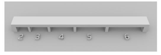
Minimum Hole Diameter and Engraved Detail Width, Z-axis, at
