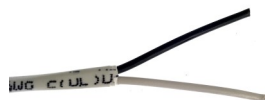
"002360-1000" BCG Blue Ridge Technology OUTPUT Signal, 18/2 18 AWG 2 Conductor Bare Copper, Non-Shielded Plenum UL Listed C(UL)US CMP White Jacket, 1000'
