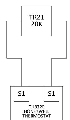
Set thermostat for Commercial Application. Indoor Sensor = 20K
