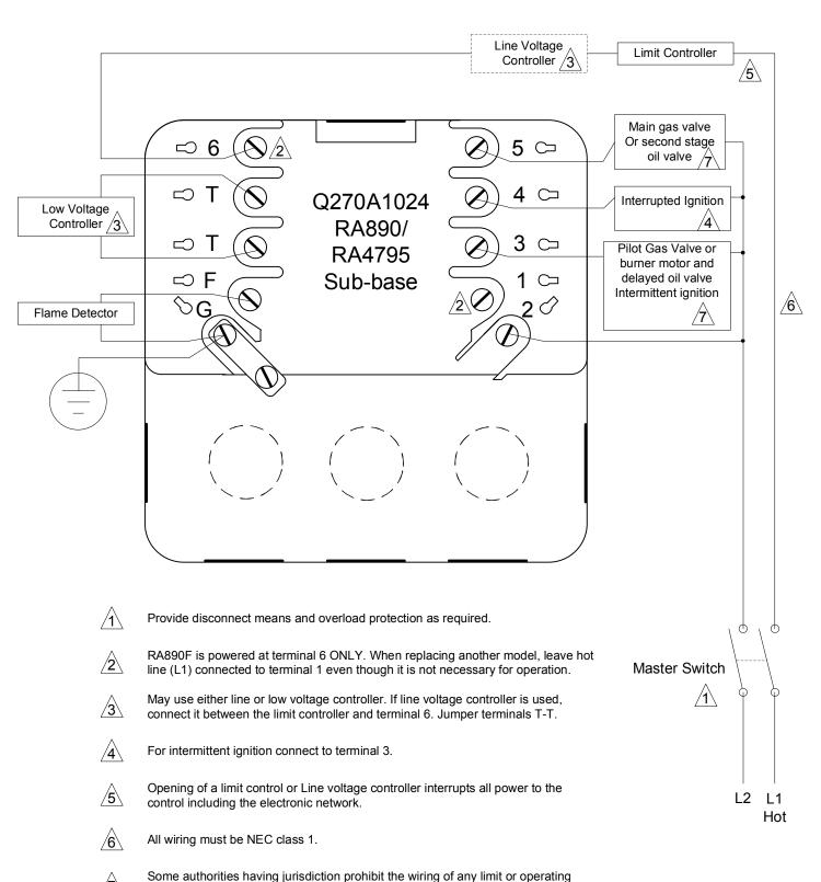
contacts in series with the main fuel valve(s).
