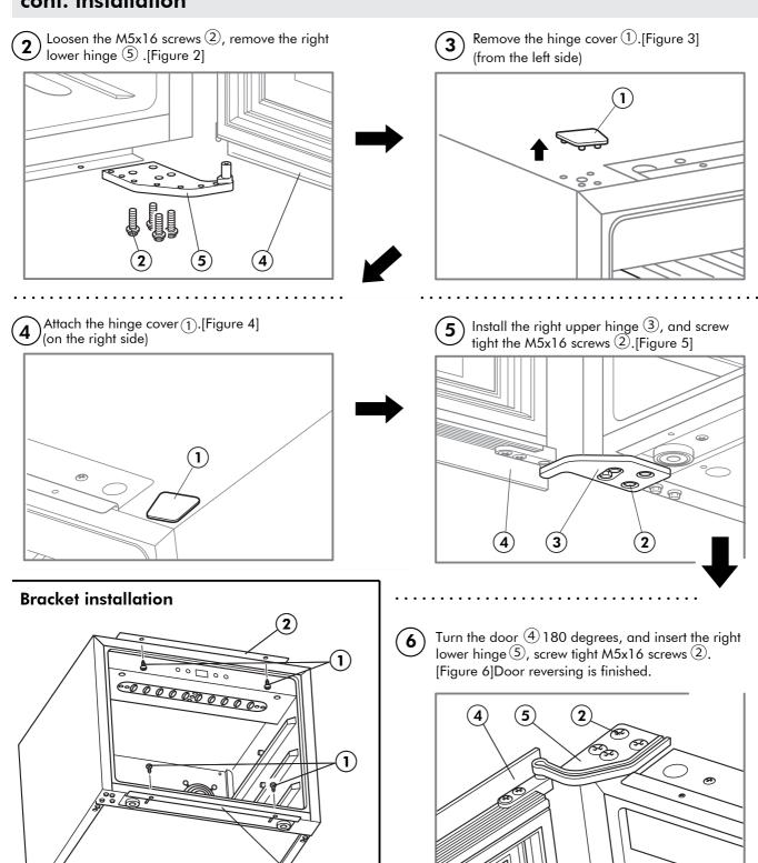
The appliance is equipped with a pair of brackets at the top (2) and at the bottom. This pair of brackets might not necessary depending on your installation situation when attaching your appliance in a closet. If the opening of the closet is bigger than the appliance, you could fix 4 screws (1), ST4x13) (packed separately in a plastic bag) into the inner wood plate of closet. In this way, the appliance will be built-in and fixed tight with your closet.
