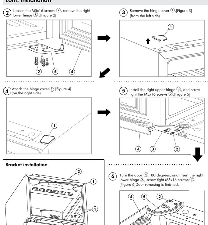
The appliance is equipped with a pair of brackets at the top (2) and at the bottom. This pair of brackets might not necessary depending on your installation situation when attaching your appliance in a closet. If the opening of the closet is bigger than the appliance, you could fix 4 screws (1), ST4x13) (packed separately in a plastic bag) into the inner wood plate of closet. In this way, the appliance will be built-in and fixed tight with your closet.
