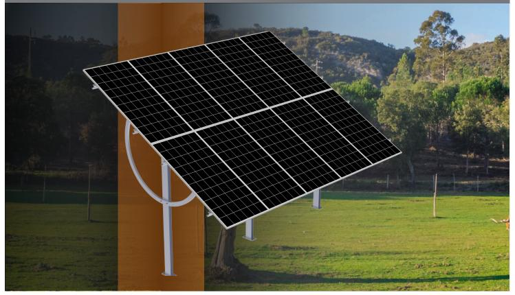
The Elios Terra G10 is a robust ground mount system designed to support up to 10 solar panels. Built from hot-dip galvanized (HDG) steel, it ensures long-lasting durability and reliable performance in all weather conditions. The system allows for quick tilt adjustments at 25°, 40°, or 55°, optimizing solar efficiency throughout the year. Easy to install and engineered for maximum stability, the Terra G10 is an ideal solution for residential, commercial, and off-grid applications.
