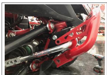
soft blow hammer so they slide over the sway bar mount a little easier. Remove the loose factory bolts on the top mounts and install them through the bumper brackets, through the sway bar mount into the frame. Now loosen the lower bolts and rotate the bumper down and back to line up the lower mounts. Install the factory bolts and tighten all four to 28 ft lbs.
