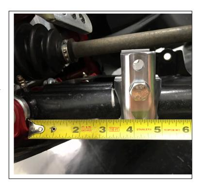
Step 7: Grab your sway bar links and install the stainless steel spacers in the rod ends. These are a tight fit and install nicely if you have them perfectly straight in the rod end. Using the 3/8" bolt in the kit, install one end of the link on the outside of the sway bar on the last
