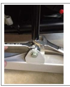
a ¾" wrench. (picture to the right) Tighten all four jam nuts. Typically you will never adjust these links. The only time you would change them is if you are running a race where your only turning left. Then you could pre-load the bar one direction or another by changing the length of the links from side to side. For 99% of off road use, the links will be the same length on both sides. You are now done with the installation!
