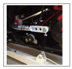
on using the longer of the two factory bolts. Do not use the large gold washer. If it does not line up then just tip the RZR side to side until it does. The three holes on the sway bar control the stiffness of the bar and limit the body roll. The hole on the end of the bar (to the rear of the RZR) is 50% stiffer than the factory bar and is this sway bar's softest setting. The center hole is 60% stiffer and the hole farthest
