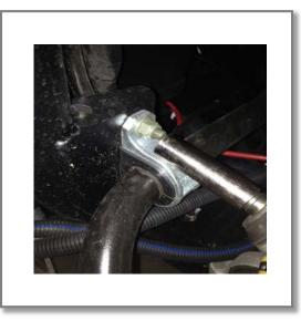
bushings are straight and not pinched in the bushing blocks. Next, install the end links. Place the spacers inside of each of the rod ends. They are tight and must be straight to be installed all the way inside of the rod end. Make sure the end links are the same length as each other. Now install the end link with spacers in the trailing arm mount. The factory bolts are different lengths. Use the short bolt on the trailing arm mount. Place the end link on the inside of the sway bar and bolt it
