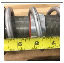
Now you can install the new upper spring. Next, install the factory plastic spring divider. Make sure the plastic divider has the long
