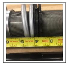
setting is 4" to the top of the upper spring. See pic on bottom of page 2. Install the mounting spacers and O-rings again. You may want to use a little grease on the O-rings because if they get dry they will squeak when you are driving.
