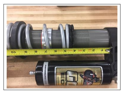
retainer down the shock shaft and out of the way of the spring retainer. With the springs loose, remove the lower spring retainer from the bottom shock mount. You can now remove the springs and the plastic spring divider from the shock.
