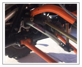
Next, install the lower part of the sway bar link to the sway bar in the loose position (hole located at the end of the bar) and tighten using a 14mm and 17mm wrench. Make sure the link is bolted to the outside edge of the new sway bar
