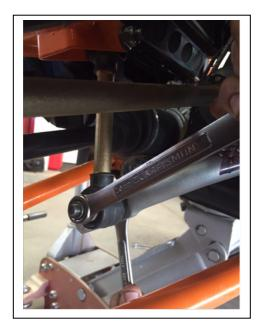
Next, disconnect the sway bar links from the sway bar using a 15mm wrench on the bolt side and a 17mm wrench on the nut side. If you purchased our billet links then disconnect the factory links from the upper arm as well.
