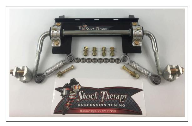
Thank you for purchasing our front sway bar kit for your RZR. This front sway bar will limit the body roll in the front of your RZR and is infinitely adjustable so that you can tune your car's ability to corner as your terrain or racing style changes.
