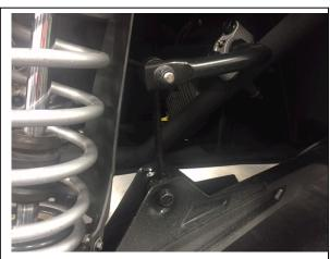
Step 3: Install our stainless steel spacers into the rod ends of your new sway bar links and install into the trailing arm using the factory bolt. Bolt the top of the sway bar link to the sway bar using the new, supplied 12mm bolt, washers and nut. This new bolt will require a 19mm socket and wrench. Repeat this on the other side of the car
