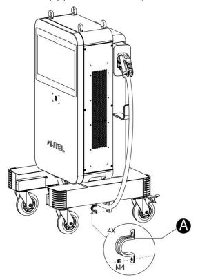
5. Remove the four lifting eyebolts and reinstall the top screws.
