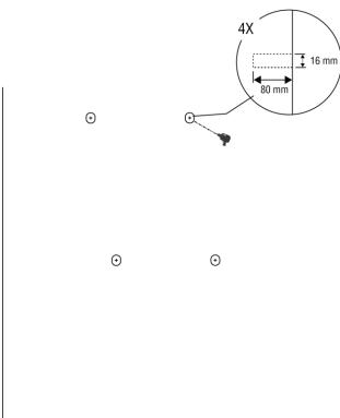
4. Tap the four M12 x 80 expansion bolts into the drilled holes. Remove the threaded bolts (**B**), spring washers (**C**), and flat washers (**D**) when the expansion sleeves (**A**) are stuck. Set them aside.
