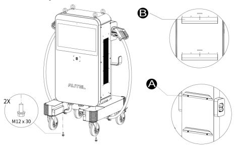
4. Use the two strain reliefs (A) (two M4 nuts for each) to secure the charging cables.
