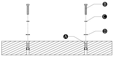
2. Loosen the four M5 x 12 screws using the T25 Torx screwdriver to remove the front cover from the pedestal. Set them aside.
