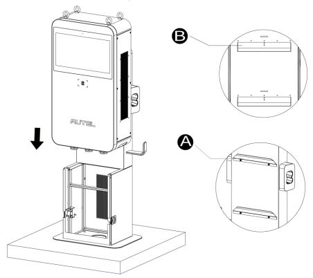
2. Insert and fasten the two M12 x 30 screws to the bottom holes (A) of the MaxiCharger using a 19 mm socket wrench to secure the MaxiCharger.
