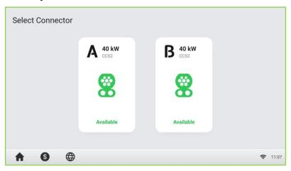
After a connector is successfully connected to your EV, the MaxiCharger can automatically recognize the connector, then the corresponding connector's Authorization Screen will appear.
