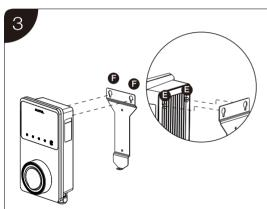
Attach the main unit to the wall dock by inserting the two protruding screws (E) on the back of the main unit into the two upper mounting holes (F). Slide the main unit downwards.
