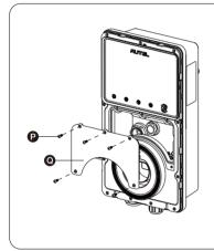
2. Unscrew the five screws (P) to remove the inner cover (Q).
