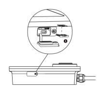
b) To connect via the SIM card, remove the SIM card cover by first unscrewing the M3 x 10 screw using the screwdriver type T10. Then, remove the SIM card adapter (I) using the pin and place the card into it. Make sure that the card is inserted correctly. Install the SIM card cover back by following procedures above in reverse order.
