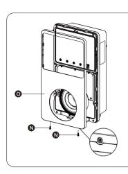
1. Remove the two screws (N) at the bottom of the MaxiCharger with the screwdriver type T10 to remove the maintenance cover (O).
