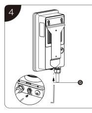
Screw the included M5 x 12 screw (G) into the hole at the bottom of the main unit and tighten the screw to secure the main unit using the screwdriver type T25.
