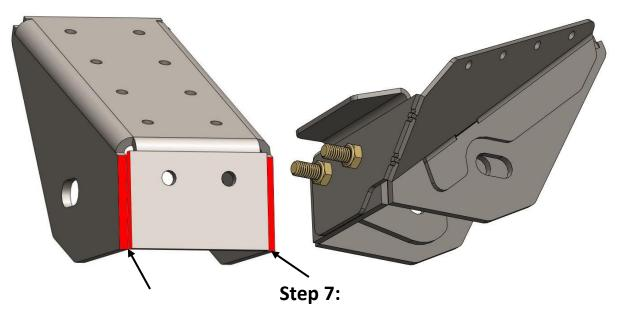
With the new gussets tacked in place, bolt the new lower control arm bracket on to the control arm. If the axle has not moved, you should be able to swing the control arm and bracket up to the frame and fit it right in place. If it seems the axle has moved, the front of the bracket should be about 2-1/16" off the cutout in the frame.
