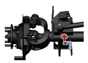
Move the flag nut in position where you can begin to thread the bolt into the nut.
