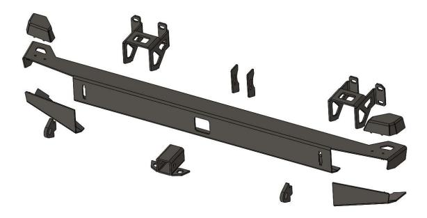
All parts will tab into the main shell. Align edges and tack weld in place.
