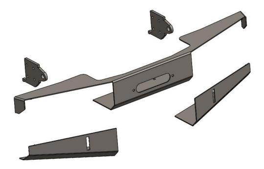
Align the bull bar and gussets with etch as shown below, tack weld in place.
