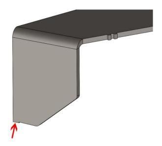
All parts will tab into the main shell. Align edges and tack in place.
