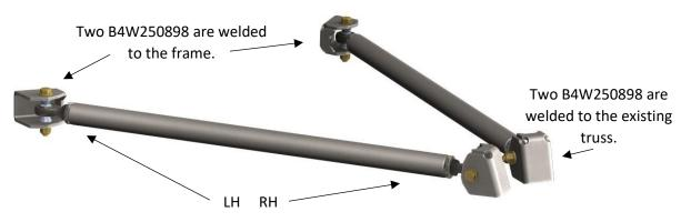
The suspension links need to contain one left hand and one right hand heim joint assembly. This will allow you to adjust the length of the link by twisting the DOM tubing once it is installed in the bracketry. A detailed view is provided below.
