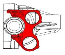
Your axle center section should look like the images below after trimming and grinding.
