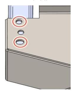
Step 6: Reinstall the factory bolts into the bottom of the bumper.
