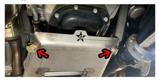
**Step 7:**Install the gusset strap and supplied hardware on the skid plate as shown below.
