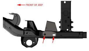
Cut the factory upper and lower control arm mounts off the frame, and grind smooth.
