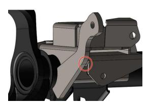
Tack weld the TJ Front Axle Sway Bar Bracket into place. Before fully welding into place bolt in the sway bar, to verify position of the Sway Bar Bracket. Once location is verified fully weld the TJ Front Axle Sway Bar Bracket into place.
