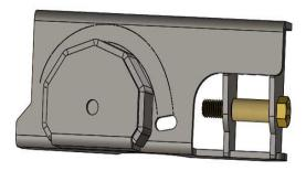
With fitment verified remove bolt and Dom Sleeve and fully weld tabs into place.
