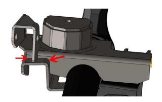
Slide the TJ Front Axle Track Bar Bracket until it makes contact with the side of the TJ Front Coil Spring Base Passenger.
