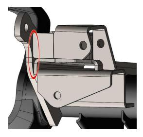
Rotate the TJ Front Axle Sway Bar Bracket on the axle until it is flush with the edge of the TJ Front Coil Spring Base Passenger. (See picture below)
