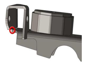
Once the location is verified tack weld the Steering Stabilizer Bracket to the Coil Spring Base Passenger.
