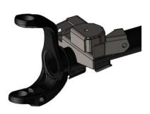
Using an angle finder position the front of the TJ Front Coil Spring Base Passenger bracket 10° back from the differential cover mounting service. Once measurements are satisfied tack weld the bracket into place.
