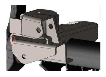
With location satisfied tack weld the TJ Front Axle Track Bar Bracket into place. Verify location by bolting in track bar. Once verified fully weld.
